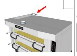
4. Flue diverter Be sure that the back flue diverter is connected firmly to the oven
